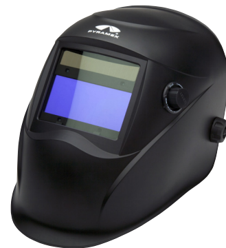
Auto Darkening Welding Helmet High-Impact Resistant Nylon Shell, 4 Independent Arc Sensors High Speed Lens - 1/30000 second Powered by Solar Cells and Replaceable Lithium-Battery Includes Magnification Lens Holder Fully Adjustable Nylon Suspension Meets ANSI Z87.1-2015
